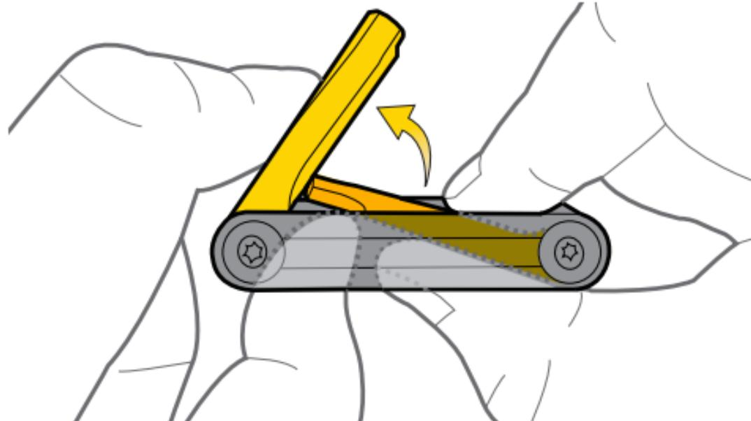
**Using both thumbs, apply force at the center of the tool to deploy it for use**
