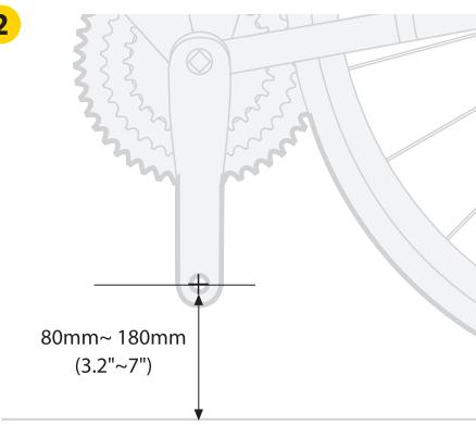
FlashStand FAT is designed to be used on bikes with crank-arm distance from the ground between 80mm and 180mm (3.2"~7").
