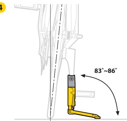
Adjust FlashStand FAT height to make sure your bike is within the recommended angle of 83°~86° (from horizontal plane) for stability of your bike. Improper installation or lean angle may cause your bike to fall and cause damage to it and/or FlashStand FAT.
