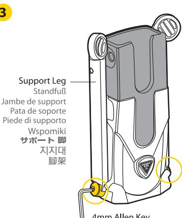
If support legs on FlashStand FAT become loose, tighten its bolts as shown. Do not over tighten the bolts as this may damage the support legs.
